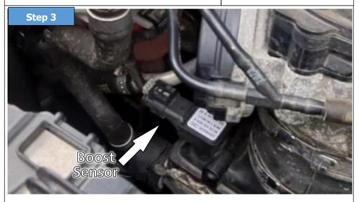
• Unplug the Boost Sensor connector (3 pin) by sliding back the grey release clip then pressing down the releasing clip and pulling back the connector.
