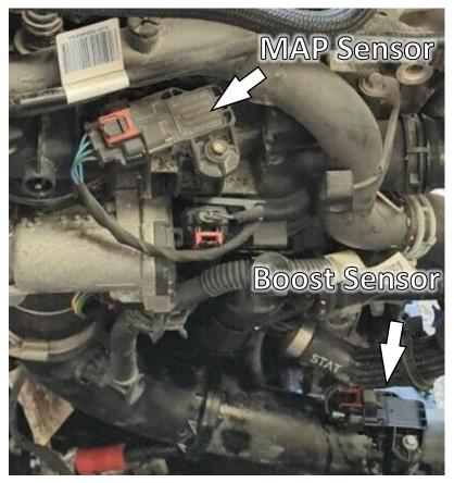
The boost sensor is located at the front of the engine on the boost pipe.
