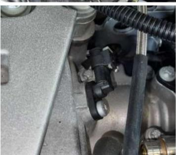
• Secure the CAM wiring loom.
