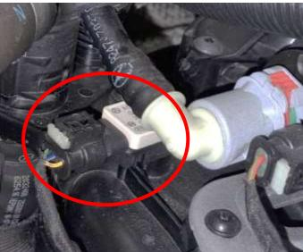
• Secure the MAP wiring loom.
