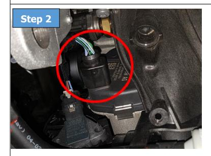
Unplug the throttle body connector by first pushing the connector forwards, pulling back the locking clip and pulling back on the connector.
