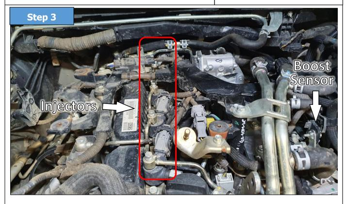
• With the chargecooler lifted, you should now have an engine that looks like the image above.
