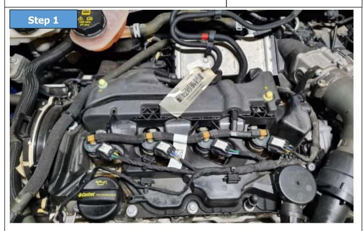
• Remove the plastic engine cover. This usually pulls off with a firm tug. On certain models the cover is secured with bolts. If this is the case, remove the bolts and lift off the engine cover.
