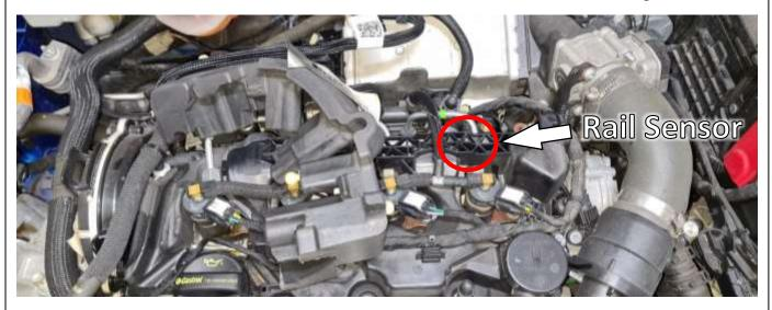
• To access the rail sensor, remove the foam injector cover. You do not need to fuilly remove the cover to gain access.
