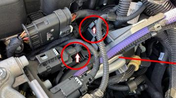
To access the boost SENT sensor, unclip the cable carrier, this is held on by two clips highlighted above
