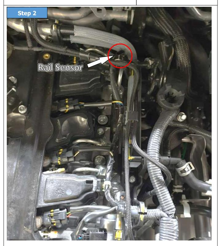
• After removing engine and injector covers you should be left with an engine that looks similar to the photo above.
