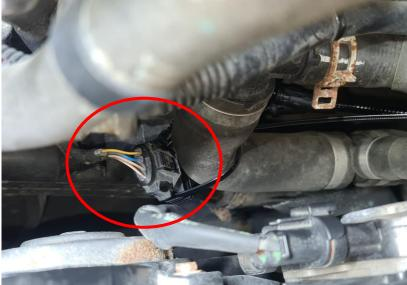
Unplug the Boost Sensor connector (4 pin) by pressing down on the releasing tab and pulling back the connector.
