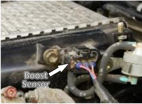
Unplug the Boost Sensor connector (3 pin) by pressing down on the releasing tab and pulling back on the connector.
