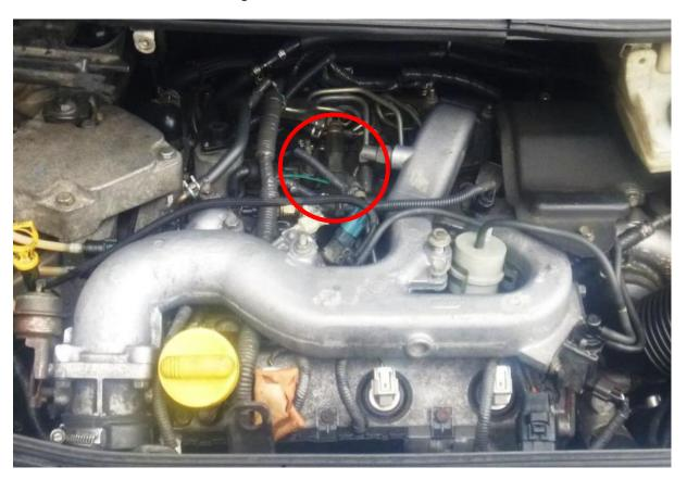
On some installations of this engine, the silver intake manifold covers the fuel rail and makes it difficult to fit.
