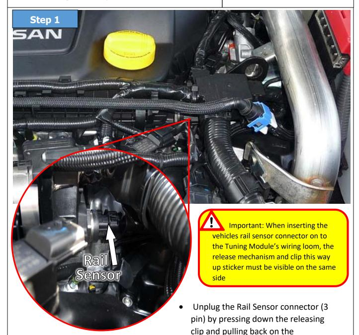
• Insert the connector from the Tuning Module's wiring loom onto the Rail Sensor. Keep in mind, that this connector can be fitted in the incorrect orientation. We have placed a "clip this way" label on the connectors for this reason.
