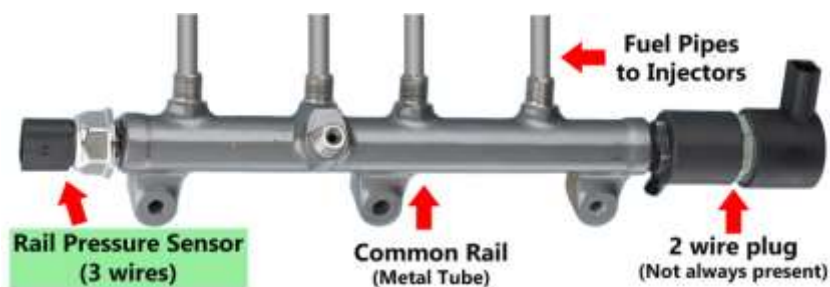
General outlook of the fuel rail in a common rail engine
